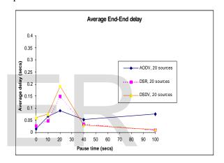
Since DSDV uses the table-driven approach of maintaining routing information, it is not as adaptive to the route changes that occur during high mobility. In contrast, the lazy approach used by the on-demand protocols, AODV and DSR to build the routing information as and when they are created make them more adaptive and result in better performance (high packet delivery fraction and lower average end-to-end packet delays).
